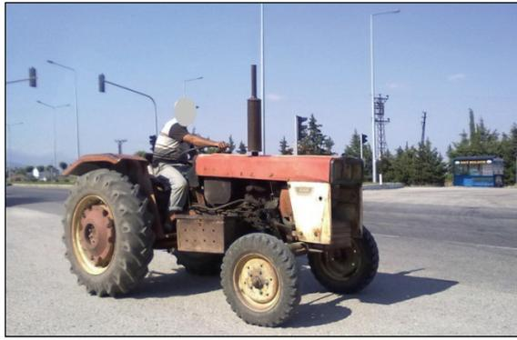
**Figure 2. Common use of farm tractors without ROPS on highway.**
