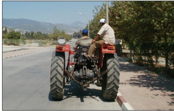
Figure 3. Common use of farm tractors without ROPS and with extra rider on highway.
